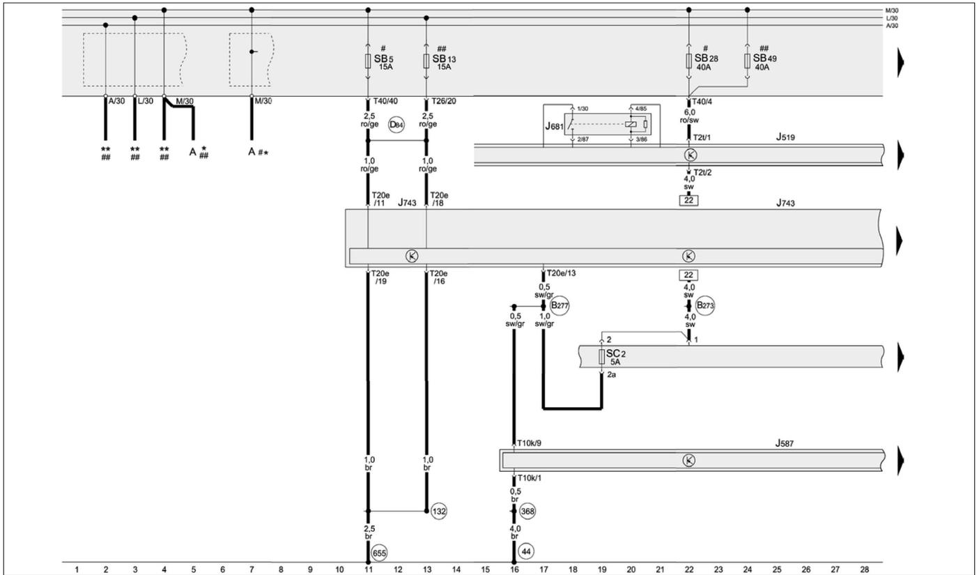
**ALIMENTATION DU BOÎTIER ÉLECTRONIQUE, FUSIBLES SUR LE PORTE-FUSIBLES, ALIMENTATION EN TENSION, BORNE 15, CALCULATEUR DE CAPTEURS DE LEVIER SÉLECTEUR, CALCULATEUR DE BOÎTE D'EMBRAYAGE DOUBLE**
