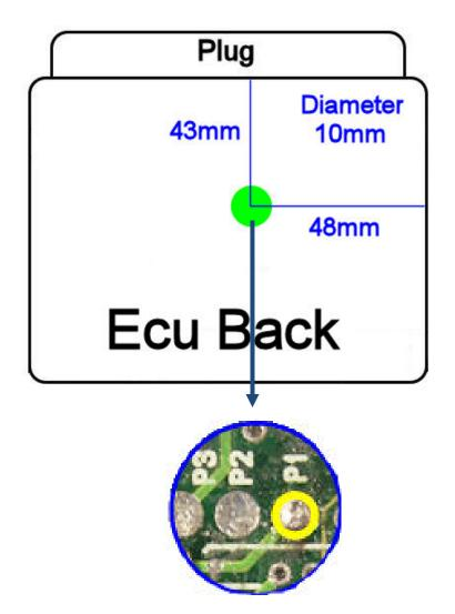
You have to connect the yellow banana of Serial Suite to P1 through the metal point. Holding connect the metal point for all time, during the connection and when you reading the Ecu. NEVER Remove the metal point for the whole procedure (Identify, Read and Write).
