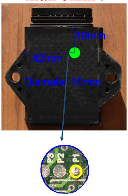
You have to connect the yellow banana of Serial Suite to P1 through the metal point. Holding connect the metal point for all time, during the connection and when you reading the Ecu. NEVER Remove the metal point for the whole procedure (Identify, Read and Write).
